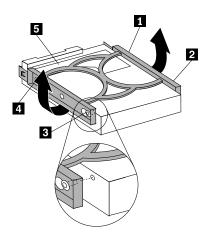
Figure 39. Installing the hard disk drive into the bracket
